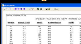
Minimum Inter Hole Spacing is 18.0 between Boreholes 2 and 3 @ depth = 2.0
